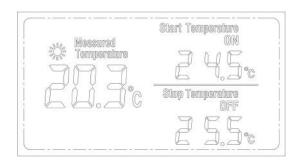
Measured Temperature lower than Start Temperature ON, the connected device is work ON; Measured Temperature over than Stop Temperature OFF, the connected device is power OFF.
