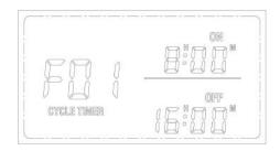
Start time delay ON, stop time delay OFF, and the Cycle timing.
