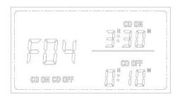
Now time is OFF, delayed (start time) ON, after starting delayed (stop time) OFF, stop the time to finish the countdown, close out the output and exit the operation.
