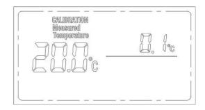
4.1 Long press FUN button, real time temperature calibration after 2 seconds. LCD first row display "CALIBRATION" and real time temperature. Correction value of LCD second row scintillation display. Adjust the correction value according to UP and DOWN button (According to the adjusted calibration value, the real time temperature changes accordingly.).
