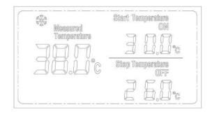
Measured Temperature over than Start Temperature ON, the connected device is work ON; Measured Temperature lower than Stop Temperature OFF, the connected device is power OFF.
