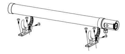
**Step 2.** Fix the tubular heater on the wall or on the floor like the following picture shows.
