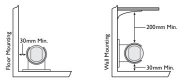
**Step 1.** Install the bracket as the picture shows.
